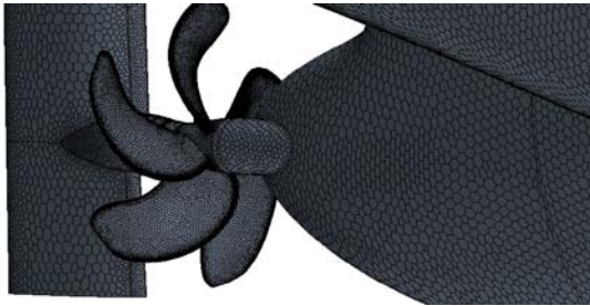
Figure 3. Typical computational mesh
