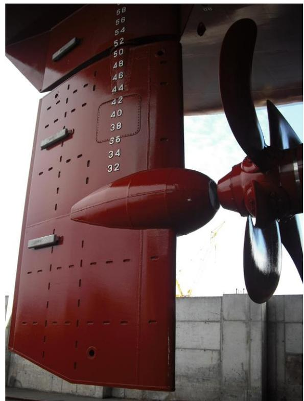
Figure 10. Twisted rudder installed on ship. This simple approach reduced fuel consumption by 4%
