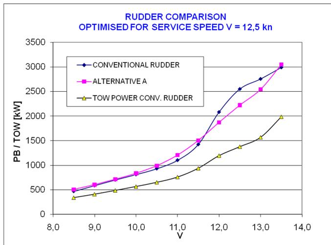
Figure 8. Power reduction on a multipurpose cargo vessel by using a tuned rudder designed by VICUSdt
