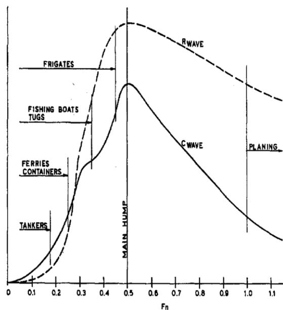
Figure 6. Typical wave resistance components
