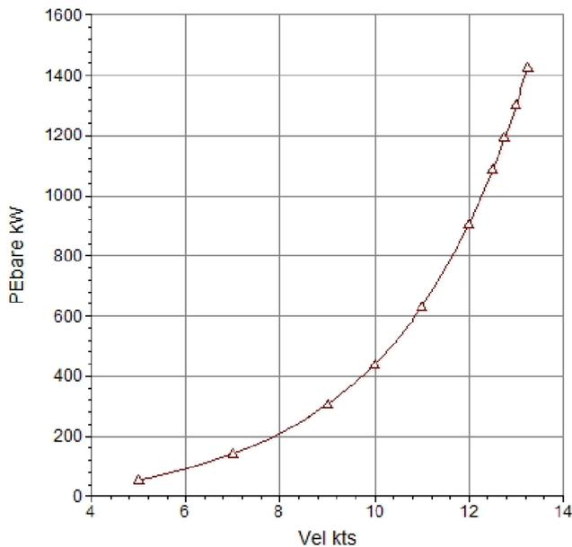
Figure 5. Power-speed curve
