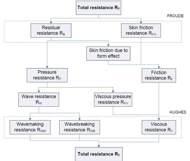
Figure 4. Resistance components
