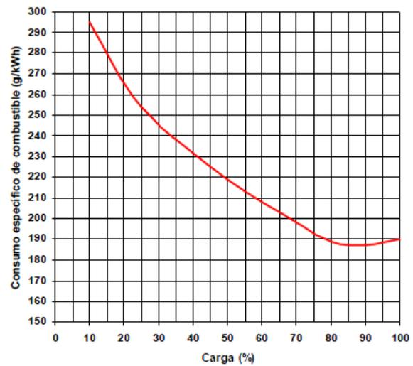
Figure 2. Specific consumer graphics depending on the load on DG sets.
