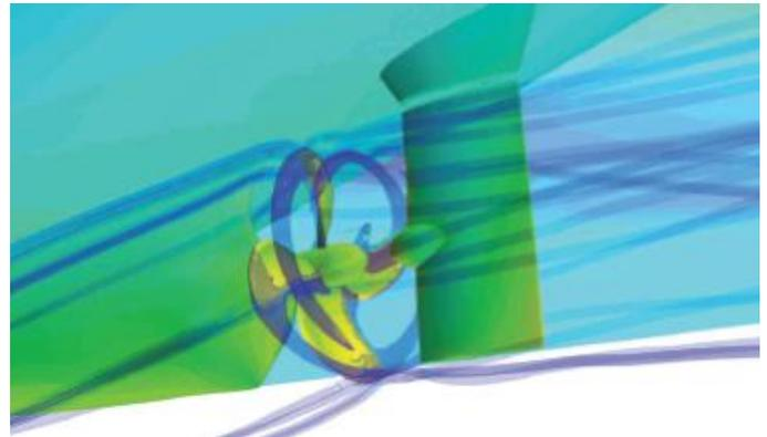
Figure 9. Rudder propeller interaction
