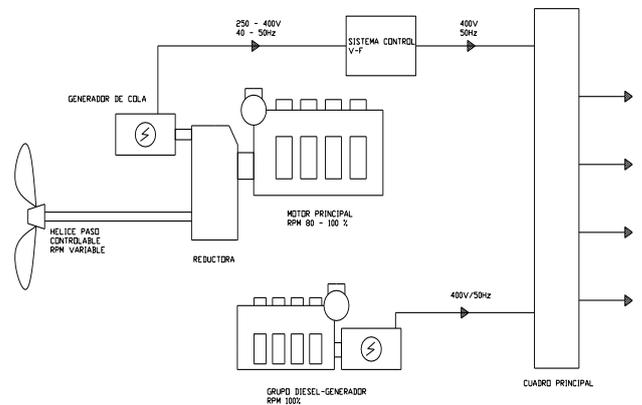
Figure 3. SHYMGEN System allows the main engine to drive a shaft generator at variable speed.
