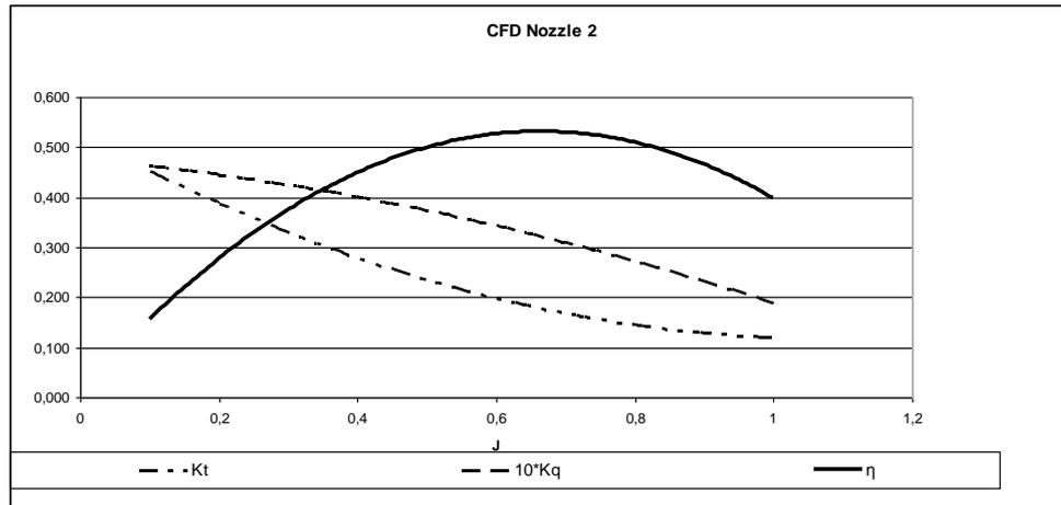
Fig. 10. CFD Results for Nozzle 2
