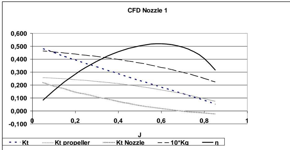
Fig. 6. CFD Results for Nozzle 1
