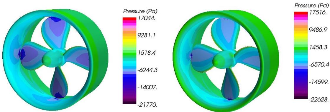
Fig. 7. Pressure distribution for  $J=0.2$  and  $J=0.5$
