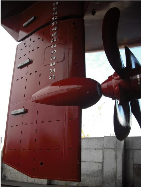
Fig. 5. Twisted rudder designed by VICUSdt fitted on a vessel.
