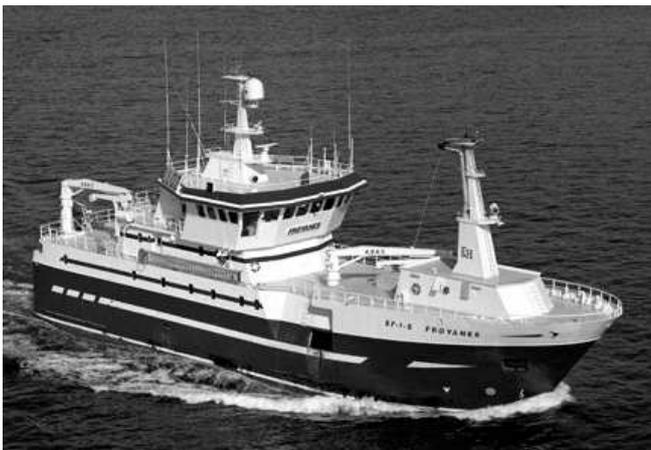
Figure 2. Diesel-electric bottom longliner Froyanes
